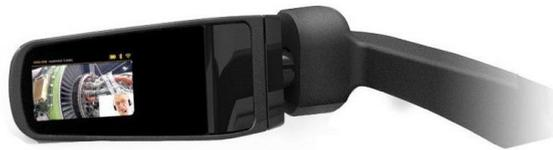
This small display shows the actual HD camera feed, or the information that the contact person on site wants to share with the field engineer who is wearing the glasses. The smart glasses can be controlled by voice commands.
