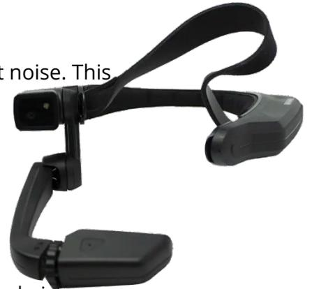
In addition to the internet, the HMT-1 needs software. To date, we have tested XMREALITY 6, HP-e MyRoom, Teams Preview, Teamviewer Pilot and Remote Eye software packages. In all situations, the device is logged on via the application to a server, which hosts the streaming from the device and distributes it to the attendees and vice versa.
