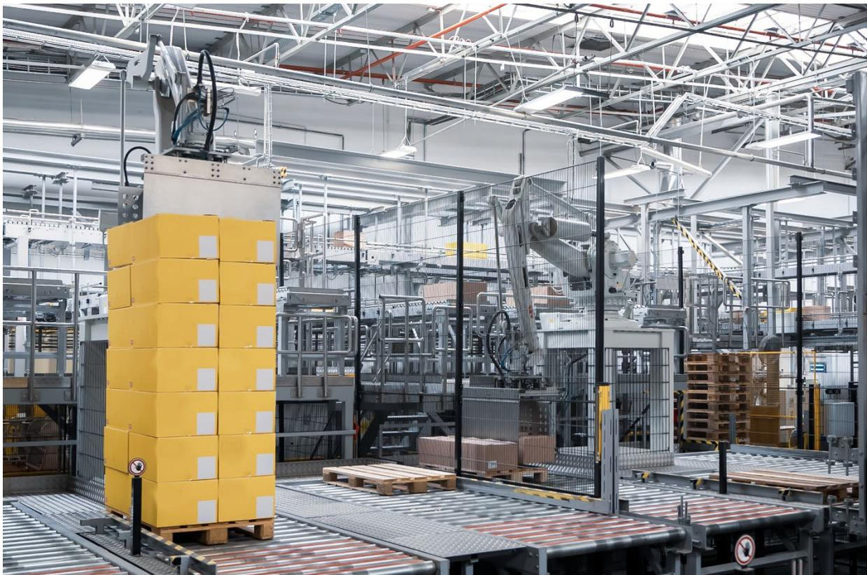
The number of cases going into a palletiser is typically 5 to 10 times fewer than the number of primary packages going into a secondary packaging machine. Whereas secondary packaging is typically organised per production line, palletising equipment is frequently chosen to handle products across multiple lines. In that case, capacity calculations have to be made for different production scenarios, taking into account sufficient buffer spaces.
